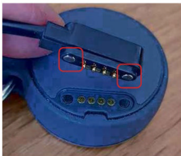
The Curve uses a non-standard USB charging cable, which connects using magnets
